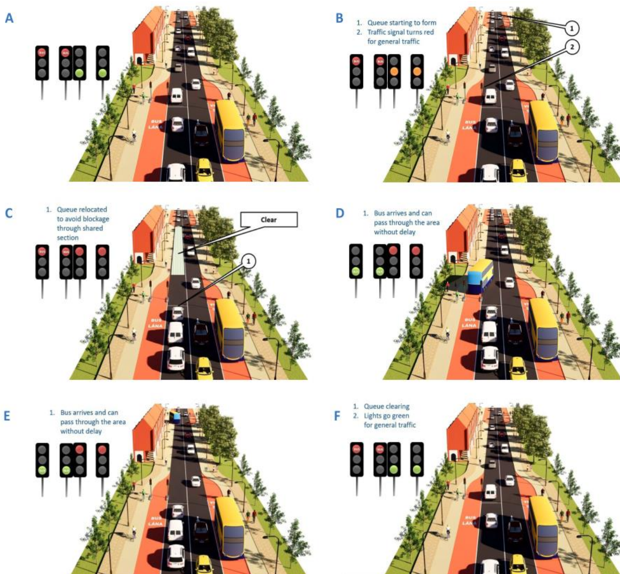
Image 4.15: SCP Schematic Operation (PDGB in Appendix A4.1 in Volume 4 of this EIAR)
